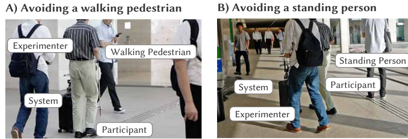
Fig. 5. User study of a real-world environment. Participants walked on tactile paving while avoiding a walking experimenter (A) and a standing experimenter (B). One experimenter crossed the participants' path at two points and blocked the path at one point.
