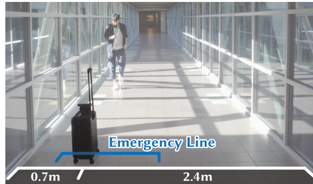
Figure 5.3: The suitcase-enclosed system in a corridor, equipped to emit various types and timings of beep sounds.
