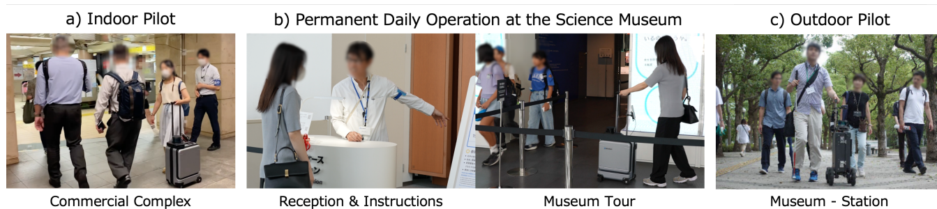
Figure 1: Field trials were conducted using AI Suitcase , an autonomous navigation robot designed for blind and visually impaired individuals: a) pilot study at a commercial complex; b) permanent daily operation at a science museum; and c) testing an outdoor model.
