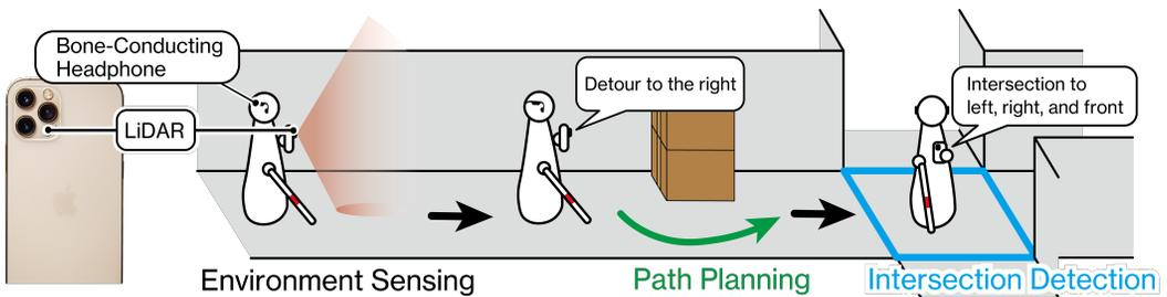
Fig. 1. Corridor-Walker assists blind people in recognizing obstacles and intersections. The blind user can use the system to detect an upcoming intersection and recognize the paths it leads to, while also avoiding obstacles.
