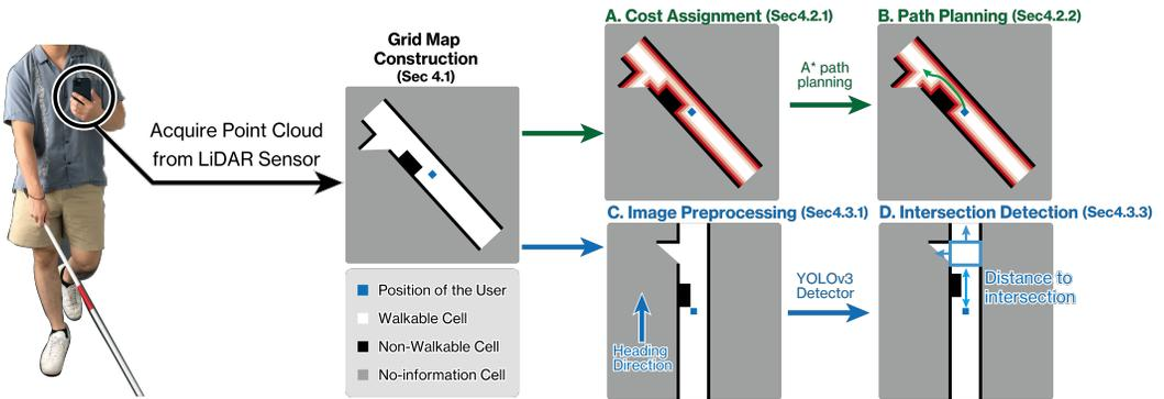
Fig. 2. Overview of Corridor-Walker. First, the system constructs a 2D occupancy grid map from the point cloud acquired from the LiDAR sensor (Section 4.1). A) Then, the system assigns a cost value to each cell (Section 4.2.1), and B) plans an obstacle-avoiding path (Section 4.2.2). Simultaneously, the system C) preprocesses the image of the grid map (Section 4.3.1), and D) detects upcoming intersections through the YOLOv3 detector (Section 4.3.3).
